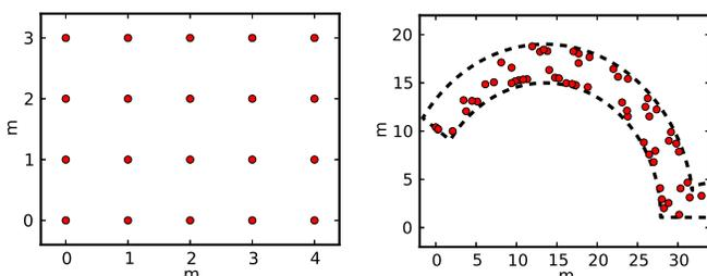
Fig. 2: Topologies of our 20-node testbed (TB-20) (left) and 60-node curved corridor testbed (TB-60) (right).
