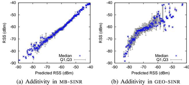
Fig. 5: **Additivity in (a) MB-SINR and (b) GEO-SINR** Correlation between predicted and measured (RSS) in TB-60.
