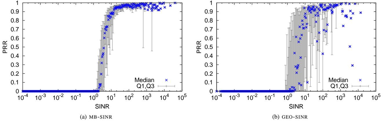
Fig. 3: **Packet reception rate for (a) MB-SINR (b) GEO-SINR.** Fraction of packets correctly decoded by receivers in TB-60 as the SINR is varied by evaluating different pairs while possibly invoking multiple senders. The plots show a phase transition between 0 to 100% PRR as the SINR grows.
