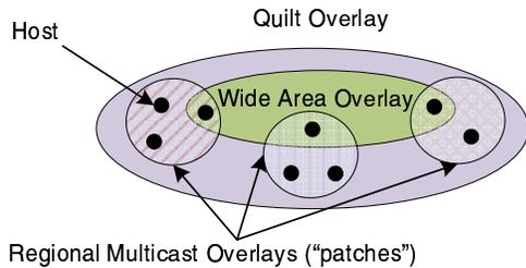
**Figure 1:** *Quilt automates the construction of complex multicast overlays. In this example, the system sews together a collection of regional multicast overlays to create a single virtual meta-overlay, separating the multicast interface from the implementation. Quilt permits the simultaneous use of various multicast solutions, each specialized for different runtime conditions.*
