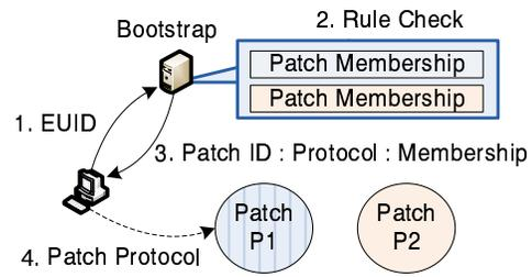
**Figure 5: Patch formation.** *Each joining host sends its locally produced EUID to the bootstrap server, which in turn finds an appropriate multicast patch (P1) for the host using various multicast rules and then returns the patch ID, protocol name and the initial membership.*
