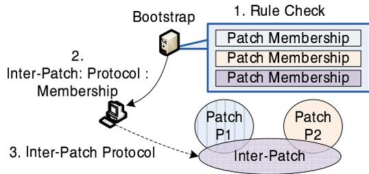
**Figure 6: Inter-patch connectivity.** *New nodes are assigned to join a regional multicast patch by the Quilt bootstrap service, along with an inter-patch multicast protocol if the patch does not have enough representatives to link to other patches.*
