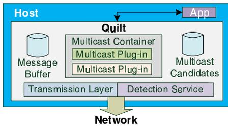
**Figure 4: Quilt architecture.** *The application treats Quilt as a single multicast overlay, but the internal structure of the system is more like an operating system supporting multiple plug-in “drivers”. In our case, these drivers are multicast protocols, each specialized for some set of conditions. Our prototype includes three such protocols: the OMNI tree, an IPMC overlay, and an ALM called DONet.*
